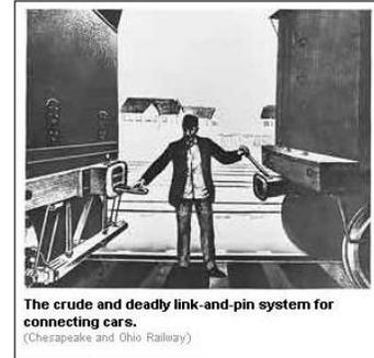
The crude and deadly link-and-pin system for connecting cars.
